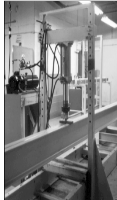
Full section bending test is conducted to assure product performance.
